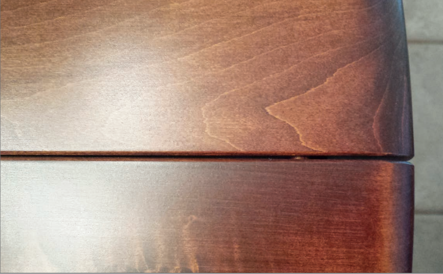
The photo above is the result of too low humidity, creating a gap at the ends of the joints. If the humidity is too high, the table will gap at the center of the joints.
